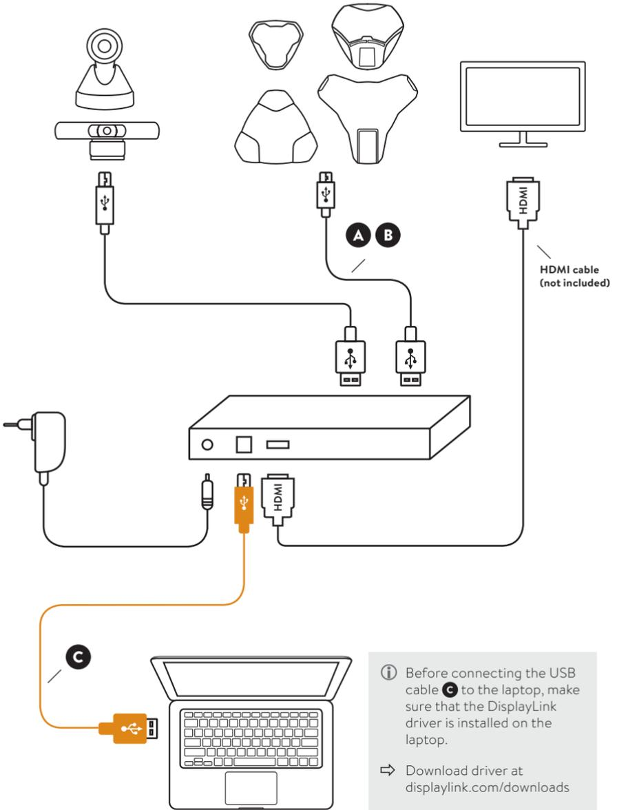
**i** Before connecting the USB cable **C** to the laptop, make sure that the DisplayLink driver is installed on the laptop.
